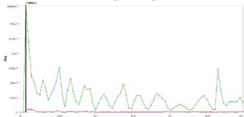
Figure 7 Maximum (green line) and minimum(red line) of the von Mises stress for 5m/s impact speed
