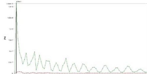
Figure 9 Maximum (green line) and minimum (red line) of the von Mises stress for 7m/s impact speed
