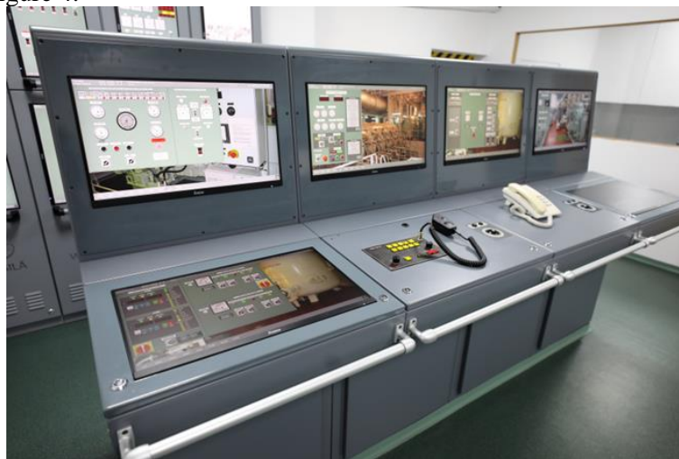
Figure 4. Main engine operating console in ERS simulator
